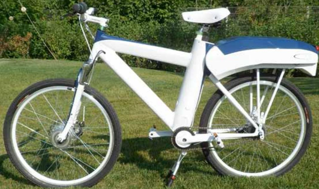
Zero emissions, pedal assist e-bike, 100% powered by hydrogen fuel-cell. Up to 300W peak power and autonomy up to over 3 hours at maximum power. All this and more thanks to H2planet solutions for e-mobility
