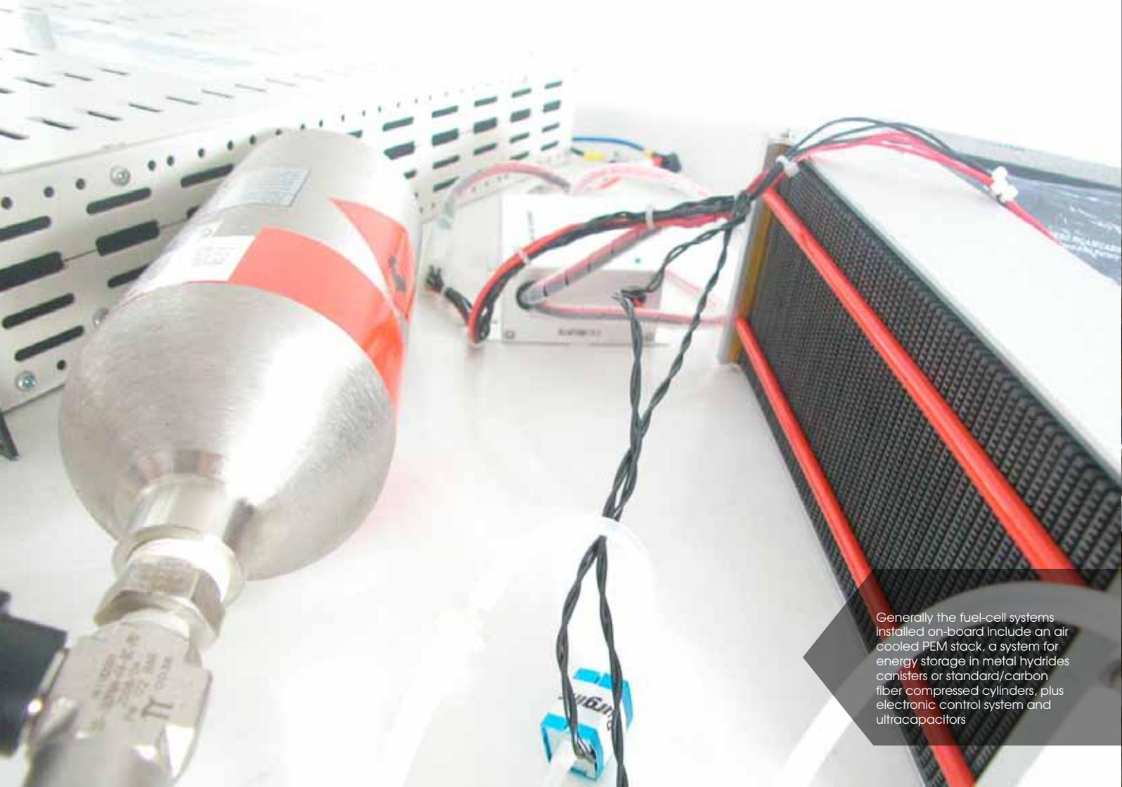
Generally the fuel-cell systems installed on-board include an air cooled PEM stack, a system for energy storage in metal hydrides canisters or standard/carbon fiber compressed cylinders, plus electronic control system and ultracapacitors
