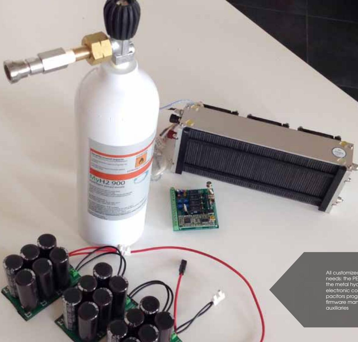
All customized according to your needs: the PEM fuel-cell stack, the metal hydrides canister, the electronic control system for ultracapacitors progressive charging plus firmware management of add-on auxiliaries
