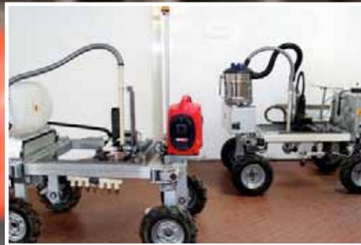
This configuration combines the latest battery technologies, or even the most traditional, in order to increase the autonomy of the vehicles up to over twice. This represents a convenient alternative to the fully fuel-cell powered configurations addressing power to recharge batteries and extending capacitance. The fuel-cell system guarantees performances that can not be compared with batteries only, allowing charging even in off-grid and stationary vehicle conditions, fully automatically.
