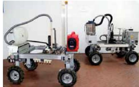
The use of H2planet fuel-cell systems on-board has doubled the range of electric vehicles
